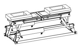
Part # Prefix & Model #: DBLG-18 Funnel Openings: 12.5 x 16.5 in. (318 x 419 mm)
