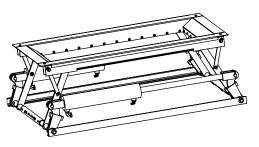
Part # Prefix & Model #: SBL-24 or SBL-30 Funnel Opening: SBL-24: 22 x 42 in. (559 x 1067 mm) SBL-30: 30 x 42 in. (762 x 1067 mm)
